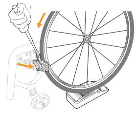
Put the cleaning cloth of MINI stick close to the drive wheel.
