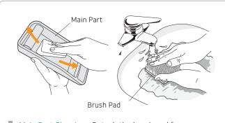
Main Part Cleaning: Detach the brush pad from the main part. Brush off dust or use tissue, etc. to clean the main part.
